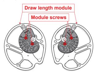
Check the following chart to know which letter fits your draw length. Make a note of the letter on the Module by the setting mark. To rotate the draw length module, you will first need to remove the two Allen head module screws. Lift and rotate the module to the desired position and replace and tighten the screws in the appropriate positions on BOTH cams.
