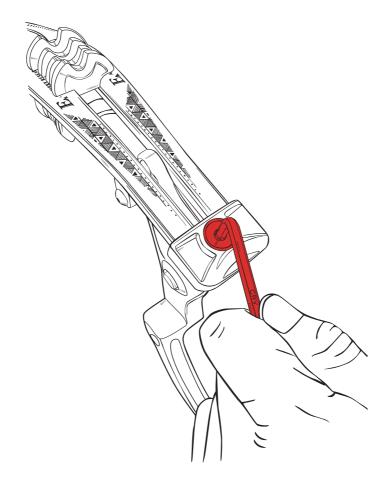
The draw weight can easily be adjusted by backing the limb bolts out (counterclockwise) on the upper and lower end of the riser. Do not turn more than 3 complete turns each time. That means when making 6 turns effort, backing the upper limb bolt 3 times, then lower bolt 3 times and then another 3 turns on each limb bolt on each side. Be sure the Limb Mounting Bolts are turned an equal number of turns to maintain proper adjustment.
