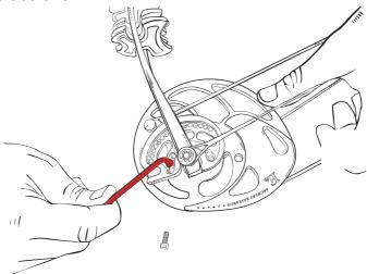
Lift and rotate the module to the desired position and replace and tighten the screws in the appropriate positions on BOTH cams. DO NOT draw the bow without the draw length module in place and secured. (Be careful to avoid over-tightening the screws, as this can strip the threads and is not covered under the warranty.)
