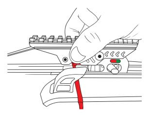
Pull the Lever back and gently cycle the trigger mechanism backwards to its original position.
