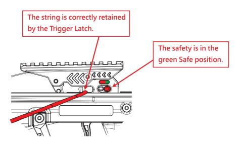
Firmly and evenly pull the Lever straight back to relock the Lever and complete the cocking of the crossbow. The Lever Lock should solidly engage the pistol grip with an audible click. (If the Lever Lock will not relock do not attempt to cock or fire the crossbow.)
