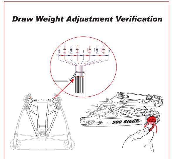
The draw weight can easily be adjusted by backing the limb bolts out (counterclockwise) on the left and right end of the riser. Always evenly back off or tighten limb bolts in quarter turns on each side. Be sure the Limb Bolts are turned an equal number of turns to maintain proper adjustment.
