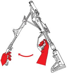
The string is correctly retained by the Trigger Latch. Note that the Safety has automatically slid backwards into the Safe position (green).
