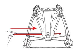
Slide the limb set into the limb slot and press it gently and firmly into place.
