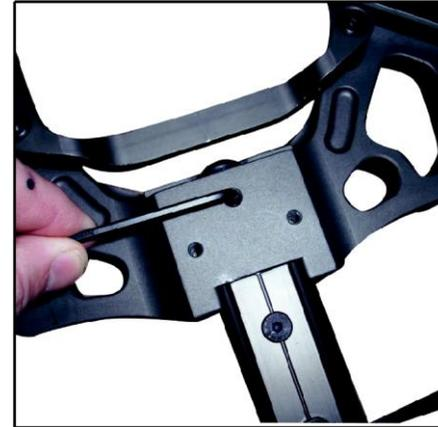
**Step 5:** Attach quiver mount found in the quiver mount hardware packet to the underside of the riser using the 2 counter sink Allen screws provided in the quiver hardware packet as pictured.
